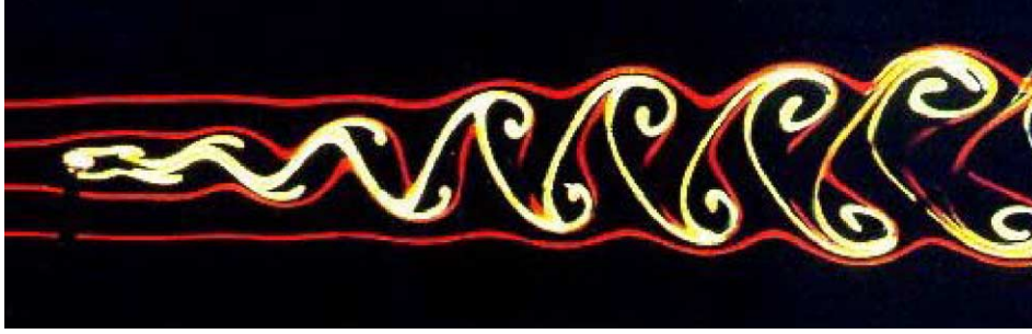
Fig. 1. Visualisation of the vortex shedding behind a circular cylinder at Re = 65 .
